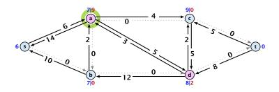
The yellow edges indicate the cut that is introduced by the smallest missing label.
