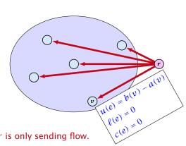
$$\begin{aligned} & \min & & \sum_{e} c(e) f(e) \\ & \text{s.t.} & & \forall e \in E : & \ell(e) \leq f(e) \leq u(e) \\ & & \forall v \in V : & f(v) = b(v) \end{aligned}$$
