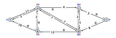
Note that the lemma is almost trivial. A node v having excess flow means that the current preflow ships something to v. The residual graph allows to  $\mathit{undo}$  flow. Therefore, there must exist a path that can undo the shipment and move it back to s. However, a formal proof is required.
