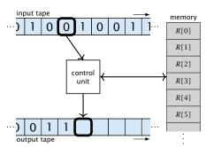
Input tape and output tape (sequences of zeros and ones; unbounded length).
