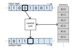
Input tape and output tape (sequences of zeros and ones; unbounded length).
