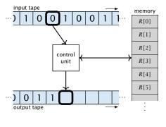
Note that in the picture on the right the tapes are one-directional, and that a READ- or WRITE-operation always advances its tape.
