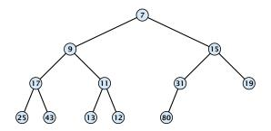
Nearly complete binary tree; only the last level is not full, and this one is filled from left to right.
