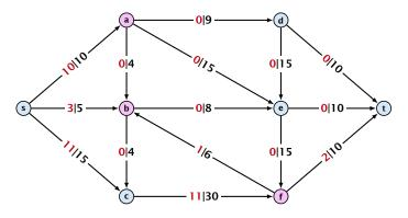
A node that has  $\sum_{e \in \text{out}(v)} f(e) < \sum_{e \in \text{into}(v)} f(e)$  is called an active node.
